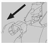
Easy to load. To remove the empty cassette, just the head guard, take hold of the cassette (see picture) and pull out.
