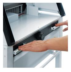
PATENTED EASY-CUT ACTIVATING BARS Blade and clamp can be activated independently via the two-step blade activating bars
